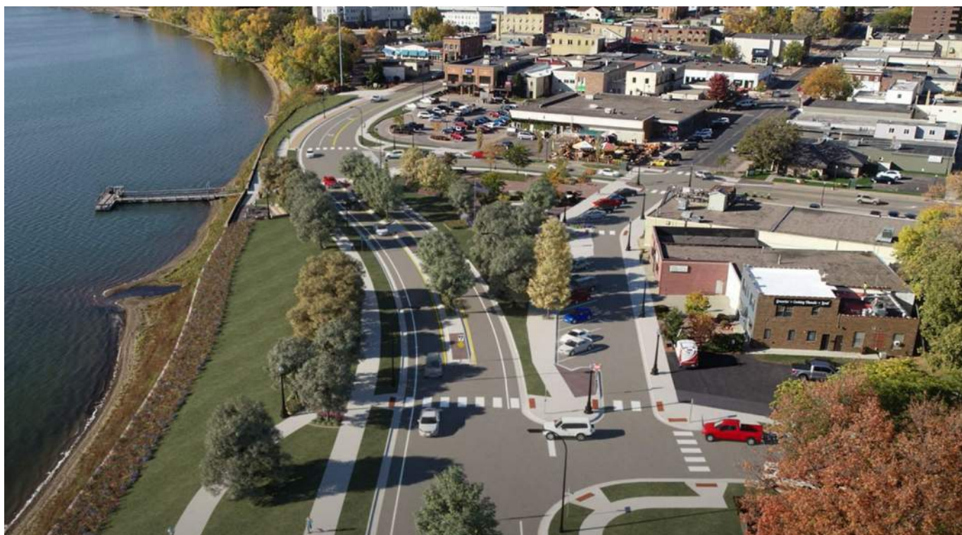
The TH 25 rebuild in downtown Buffalo will create a safer pedestrian crossing environment, re-organize parking while adding green space to the downtown splash pad, and realign traffic lanes to realize more open space at the lake edge. (Image from Bolton & Menk)
